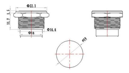
Mounting hole diameter 19mm
