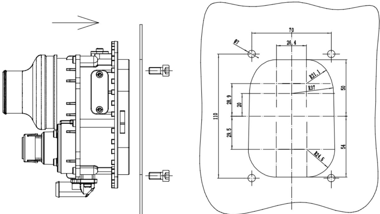
The bolts required are M6 (not supplied in the kit). The maximum mounting panel thickness is 8mm. When choosing where to place the charge port keep in mind the stop charge button should ideally also be mounted close by.
