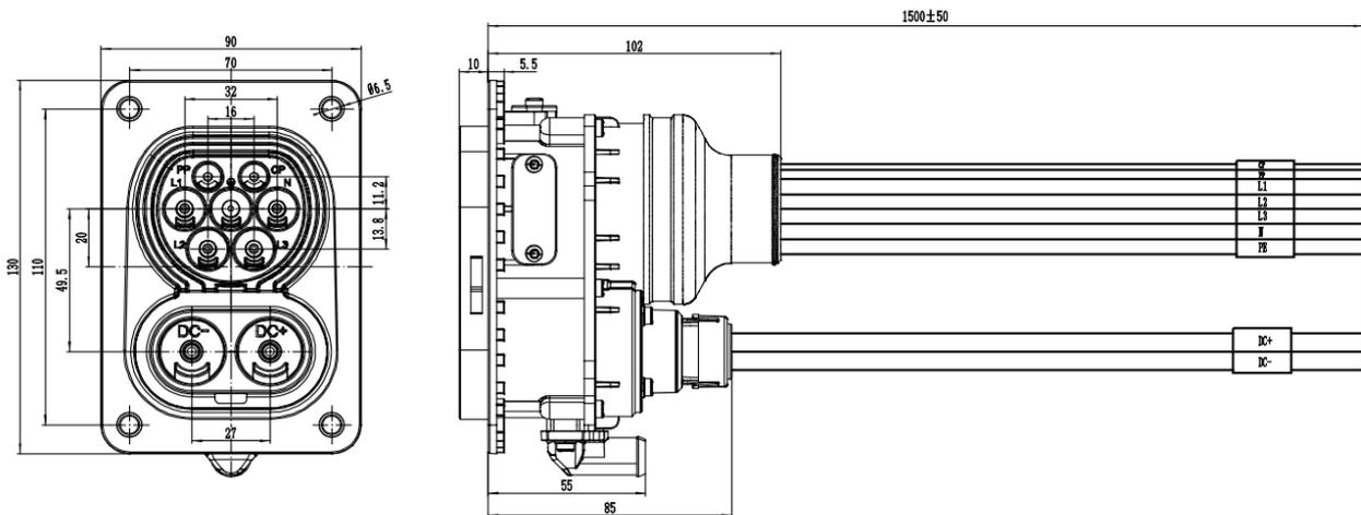
The CCS Charge inlet is significantly larger than a Type 1/2 AC Charge inlet.
