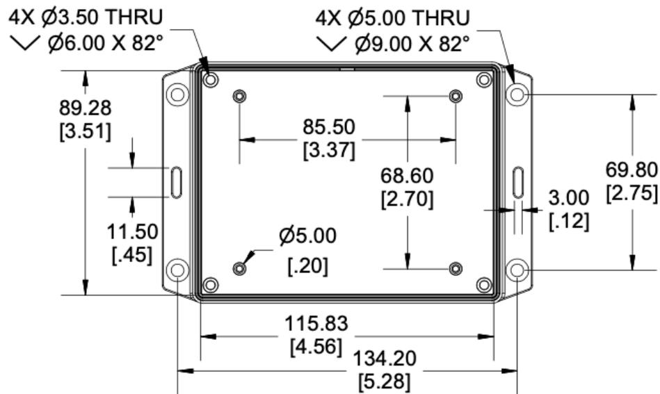
The Contactor Controller needs to be mounted inside the battery box (**It is not waterproof**). This is IP31-rated and requires HV connections. As a result, the contactor controller **should not under any circumstances be mounted outside the battery box**. It has both mounting slots and mounting screw holes.
